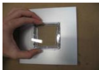
REMOVE THE GLASS FROM THE METALLIC FRAME
