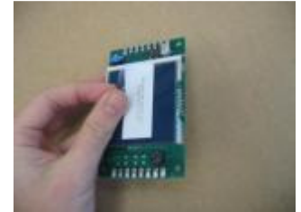
REMOVE THE PROTECTIVE FILM OF THE DISPLAY
