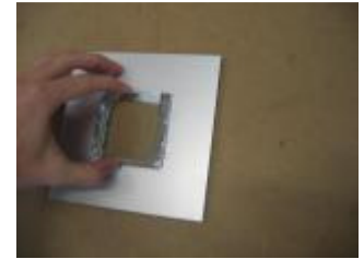
INSERT THE GLASS IN THE FRAME
