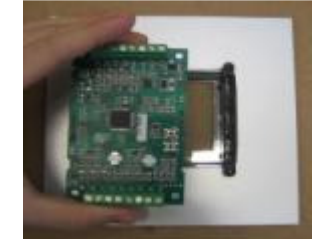
REMOVE THE BOARD FROM THE PLASTIC CHASSIS
